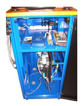
Power source, ground, and Cal Gases inlet ports from underneath access.
